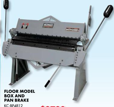
Bending length 48"Capacity 12 GaugeWeight 1140 lbs
